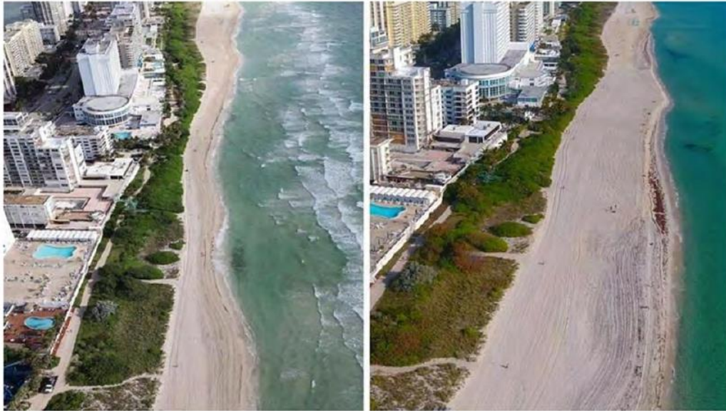
Figure C-2 Beach nourishment before (left) and after (right)
