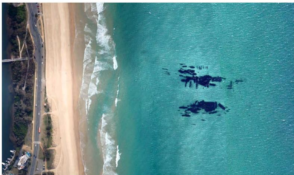
Figure 3-4 Geotextile Sand Container Artificial Reef at Narrowneck, Gold Coast (Source: NearMap, 2011)
