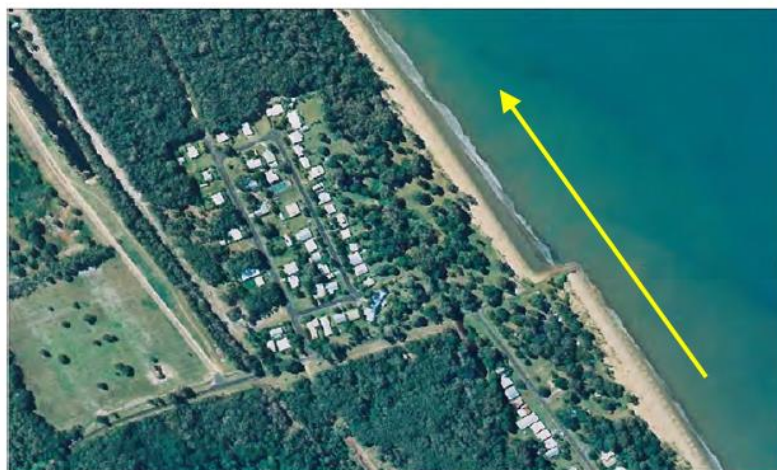
Figure C-8 Typical groyne result with longshore transport. Arrow indicates direction of sand transport
