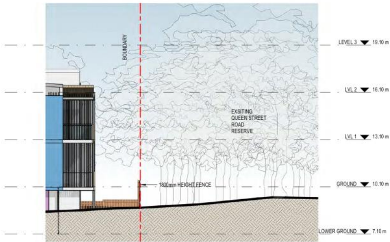
C 3.20 SECTION C - CROSS SECTION - SOUTHERN BOUNDARY 1 : 100
