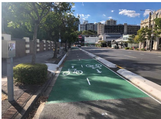
Figure 27: Two-way cycle track on Annerley Road, Brisbane
